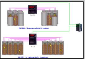
The INL150N is an monitoring unit allowing combination of a large number of temperature sensors in a single device. The « all digital » technology of the whole, reduce significantly the wiring and implementation costs, the sensors being interconnected on a 3 wires bus.
